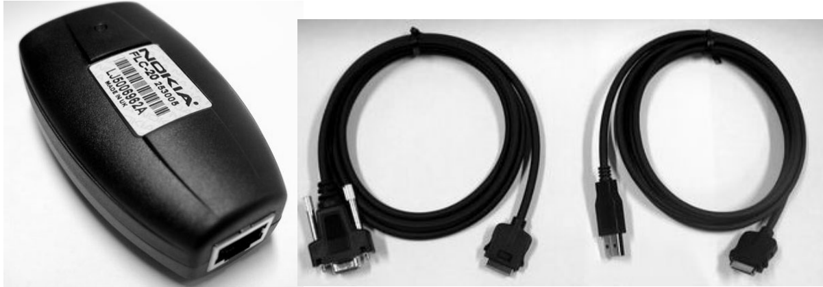
Figure 4: FLC-20 dongle (far left); Serial port cable (middle); USB port cable (far right)
